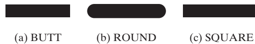
FIGURE 31.15 (a) No decoration for a BUTT line cap. (b) A half circle is added to an unclosed path. (c) A square with half of the stroke width is extended to an unclosed path.
